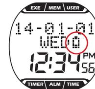
In case the power low indicator persists displaying, get the battery replaced immediately.
