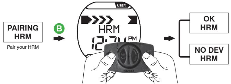
Please refer to the heart rate strap manual on wearing it properly, or press and hold the metal button at the back of the heart rate sensor (HRM) with both hands until the "OK" message prompts in your BRW.
