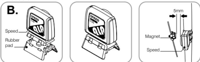
1. 1.Fasten the Speed Sensor along with the Rubber Pad and secure them on the front fork by cable ties. (ALA logo should face outward). The vertical distance should not be longer than 200 cm from Cycling Recorder.
