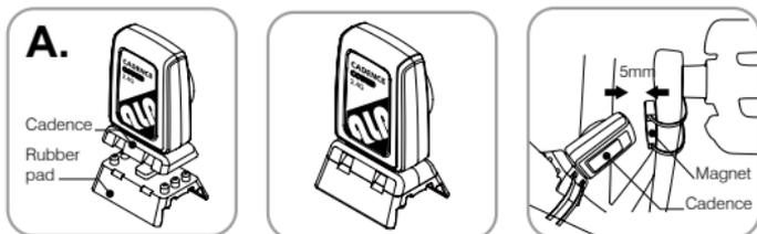
1. Fasten the Cadence Sensor along with the Rubber Pad and secure them on the seat tube or down tube by cable ties. (ALA logo should face outward.)
