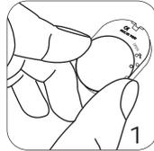
Step 2: Place the battery (type: CR2032) into the cover with positive (+) side facing the inside of the cover. Make sure the O-ring is on the cover to ensure water resistance.
